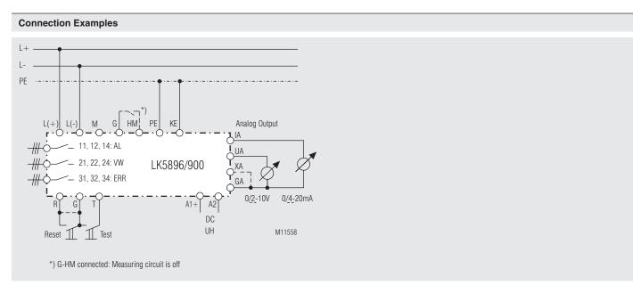
Connection to a simple DC system. When terminals HM-G are open the device triggers itself automatically.
