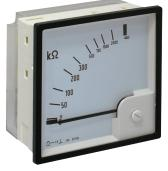
The indicating device EH 5861 is externally connected to the insulation monitor on terminals UA / GA (0 - 10 V) and shows the actual insulation resistance of the voltage system to ground. Dimensions: Width x heigth x depth 96 x 96 x 52 mm
