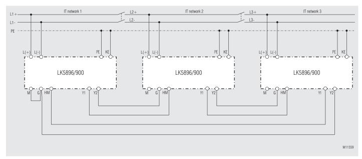
Monitoring of 3 separate DC voltage systems, that can be coupled by coupling switches. By sequential triggering of the insulation monitors it is made sure that only one of the insulation monitor is active at the same time. the first insulation monitor in IT network 1 is configured as master and starts the measuring cycle after power up.
